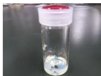
**Figure 7.** Appearance of the hybrid gel obtained from poly(NVC) hybrid star.
